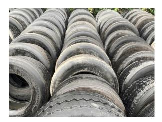
Other truck tyres that don't get taken for Casings/retreading can be regrooved if suitable, which also maximises the tyre life.
