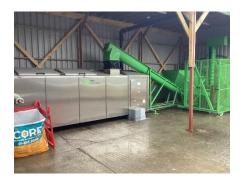
The initial focus of the project was to address the accumulation of horse stable waste. Drawing upon our expertise, we introduced our innovative aerobic treatment machine. The concept of the project was to install a trial machine at Castlerea to minimize the waste, converting it into a valuable resource to be use in the Equine Centre facility. The technology was rigorously tested and adapted to transform horse stable waste into a high-value biofertilizer.
